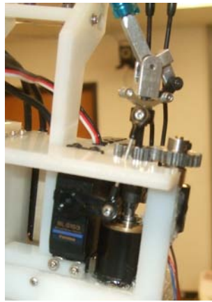
Figure 6. Close-up of amplitude controlling servo and drive shaft
